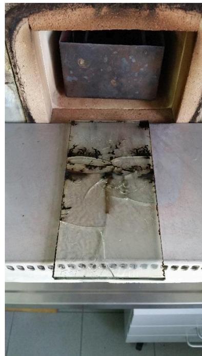
The cracking glass can be ignored, this was due to the handling of the laminated glass out of the oven.
