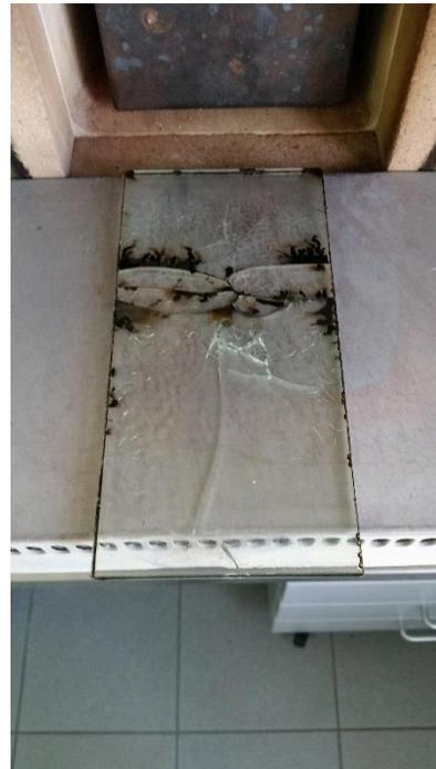
Also at 350°C, the evguard holds the laminate together.
